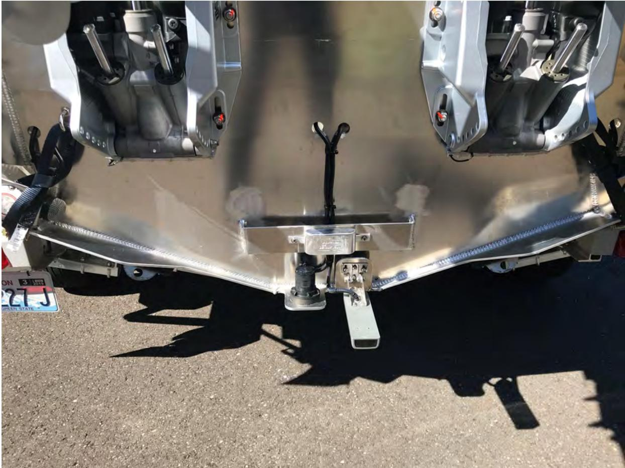
Dual transducer configuration easily adapted for ability to have a high speed chirp transducer with a side-scan transducer in combination.
