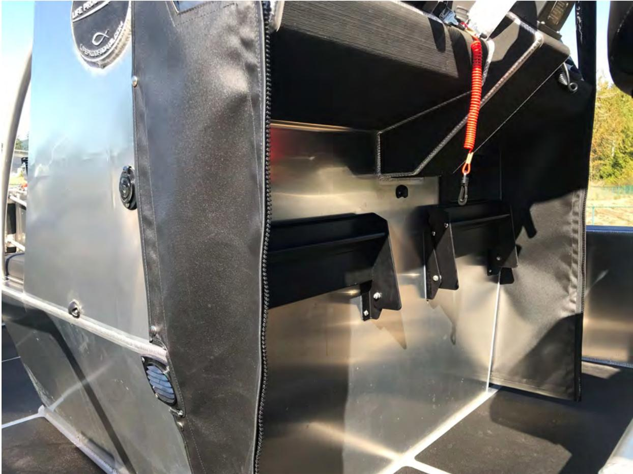
Multiple options available for footrests including these simple fold-up foot-rests mounted to the console.
