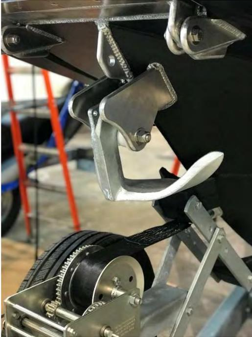
Figure 3: Bow Pulpit for Anchor
