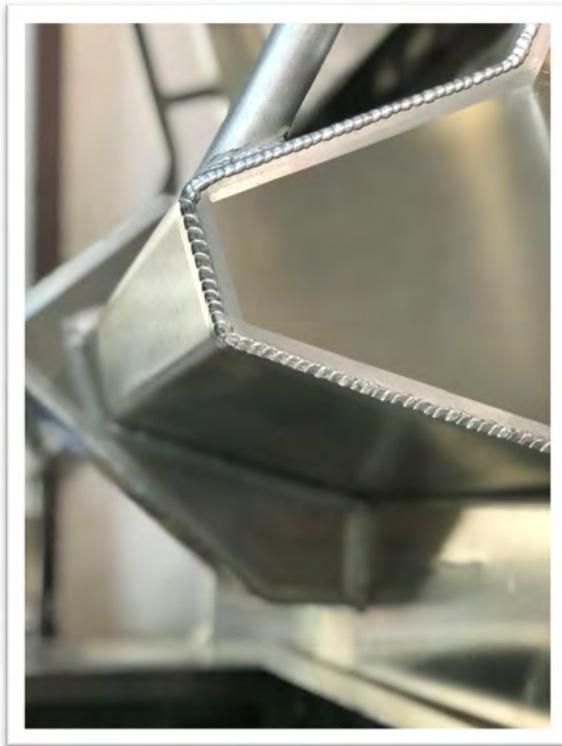
We also engineer all of the boat's structural pieces to "egg crate" or interconnect. That is to ensure a perfect fit and add rigidity to the platforms.
