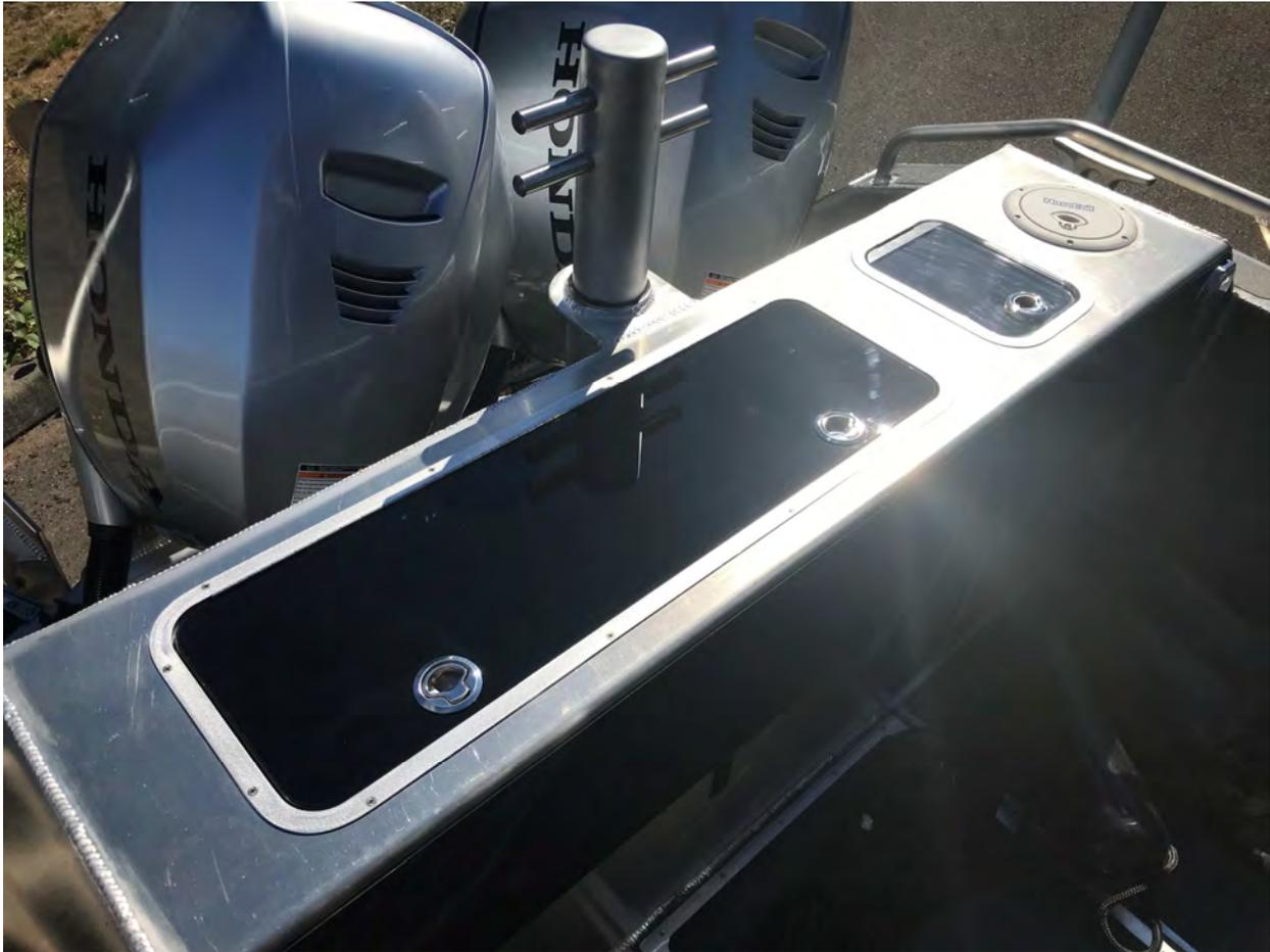
Rigging lockers are customizable in layout based on what is ordered. The lower half is typically dedicated to rigging, and the top half can be configured with storage or other options including a walk-thru transom door or a bench seat.
