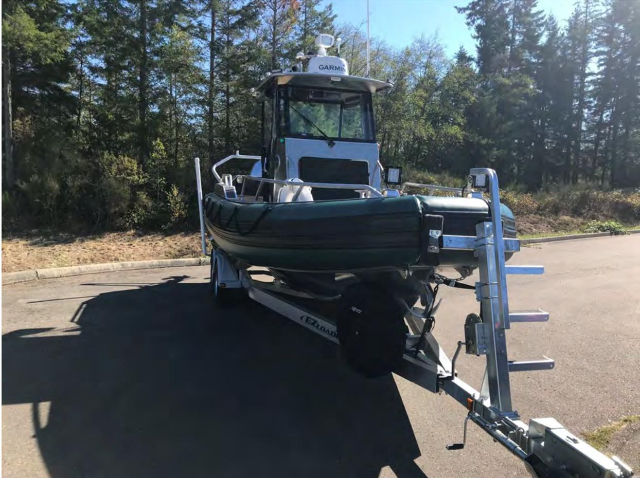
Trailer configured with bow ladder for access when launching boat.
