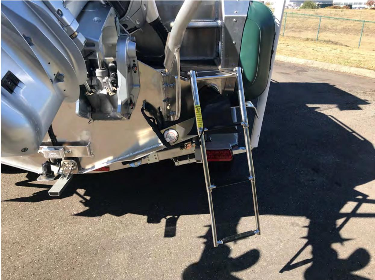
Three or Four Rung Ladder off stern swim deck for easy egress from water and or access to boat even when on trailer.
