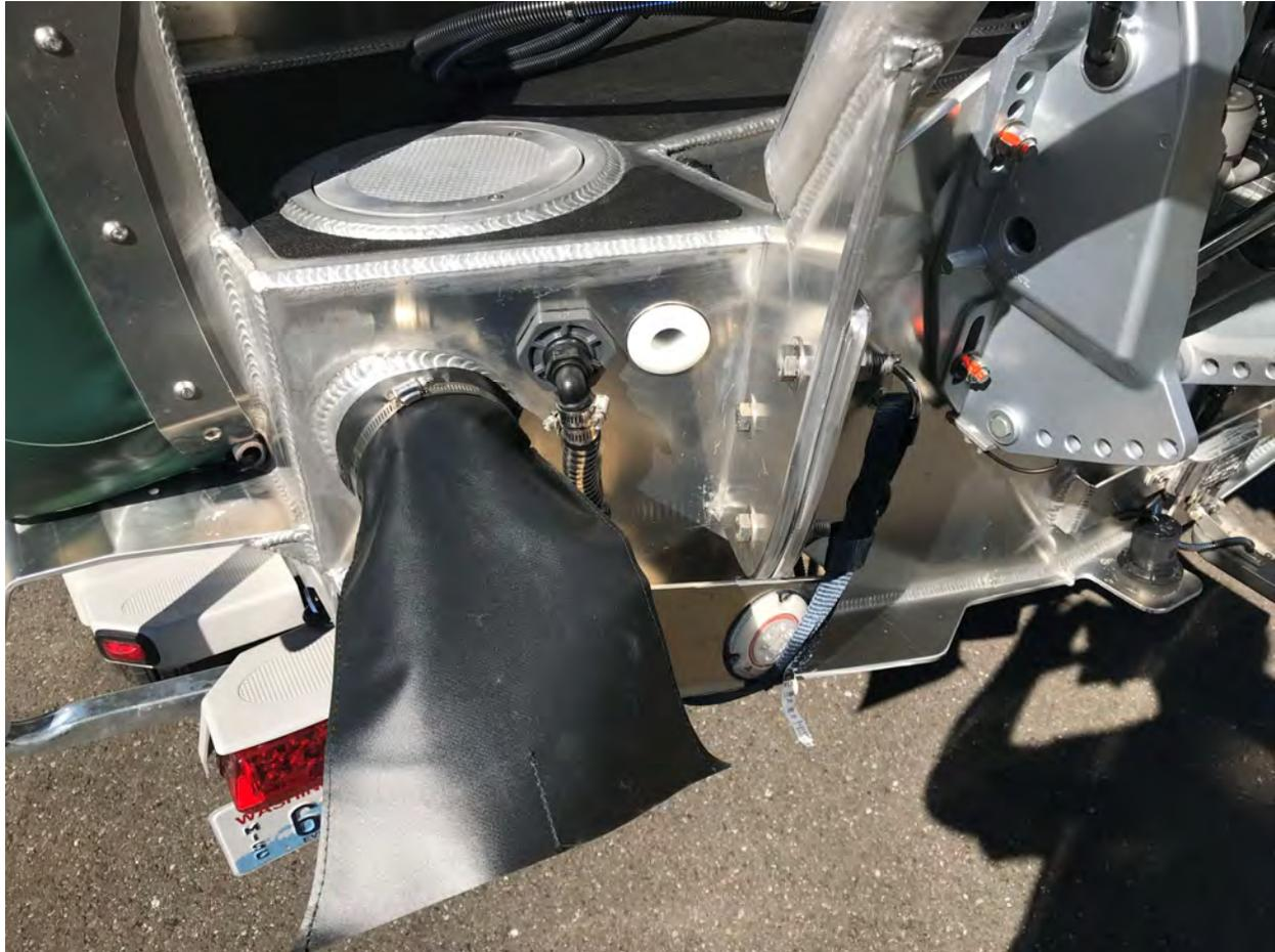
All hull penetrations happen above waterline except for a single drain plug in the boat which is below waterline. All accessories are mounted to exterior brackets / plates off transom.
