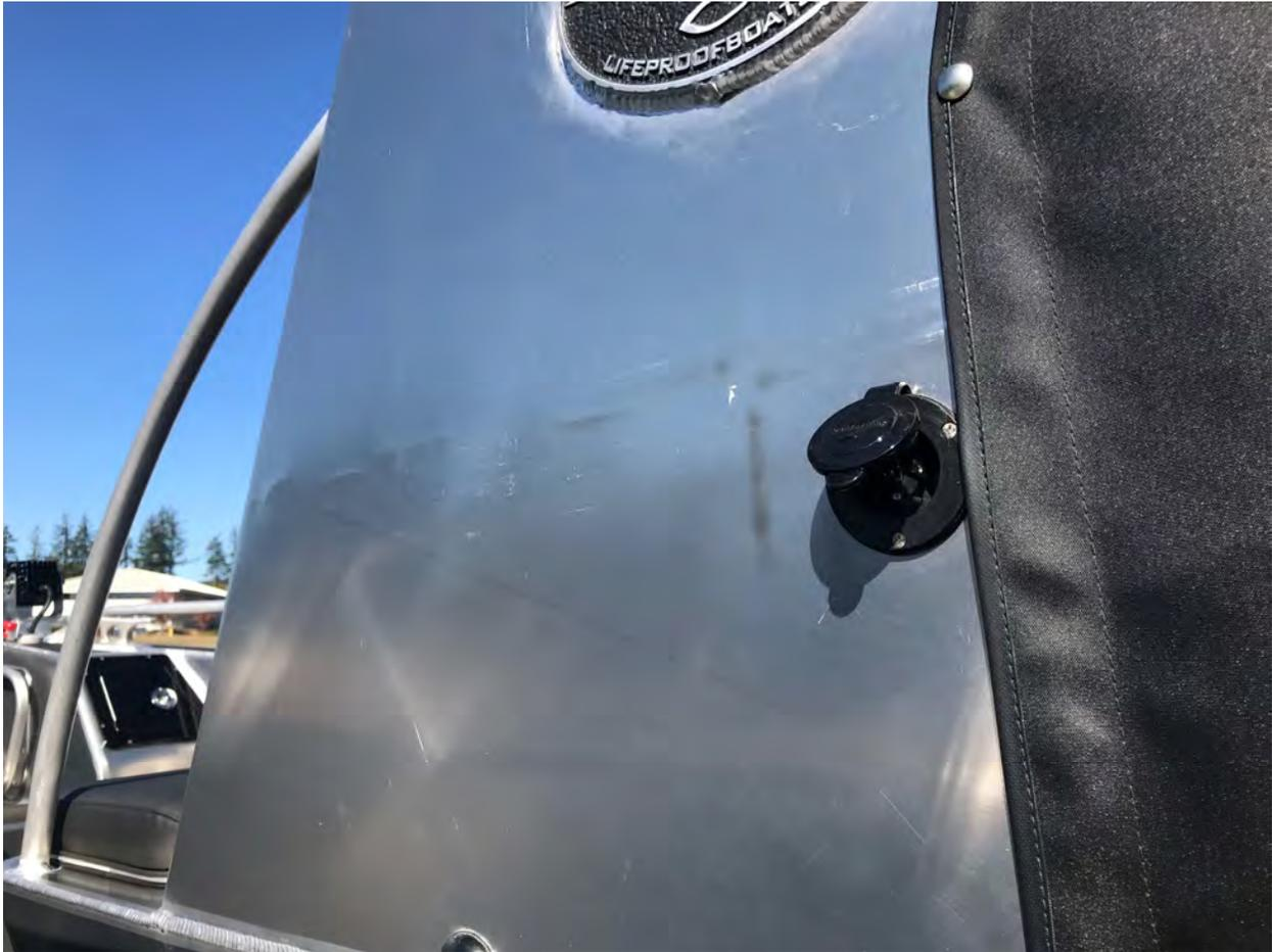
With a battery charger option, we install this simple plug on the side of the console which allows a orange extension cord to plug directly to it when the boat is stored on the trailer and you want to keep the batteries topped off.
