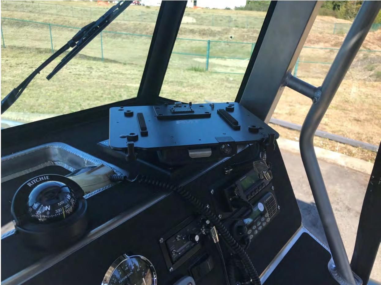
IMS manufactured a simple low-profile swivel for the above laptop docking station.
