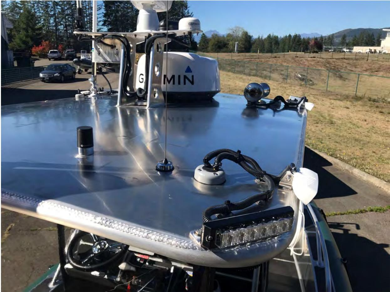
Standard in our hardtop police models is to use corner mounted LED alert lights made by CODE3.
