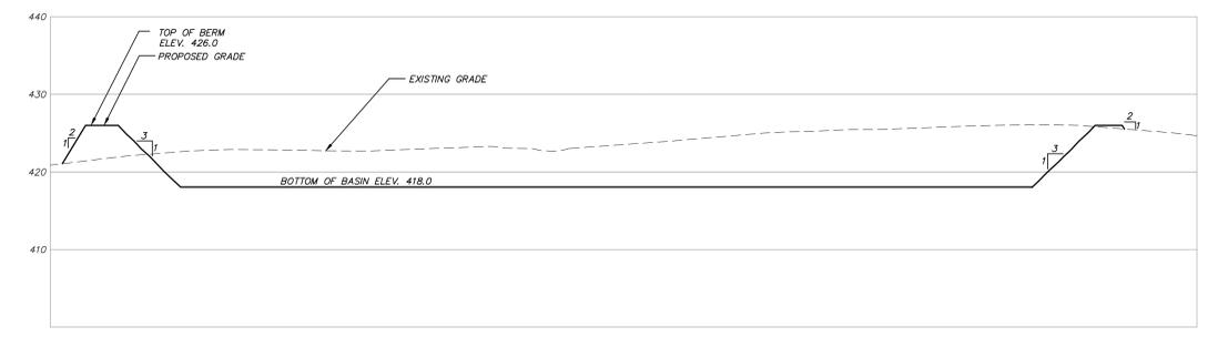
STORMWATER BASIN 2.2P SCHEMATIC SECTION E-E
