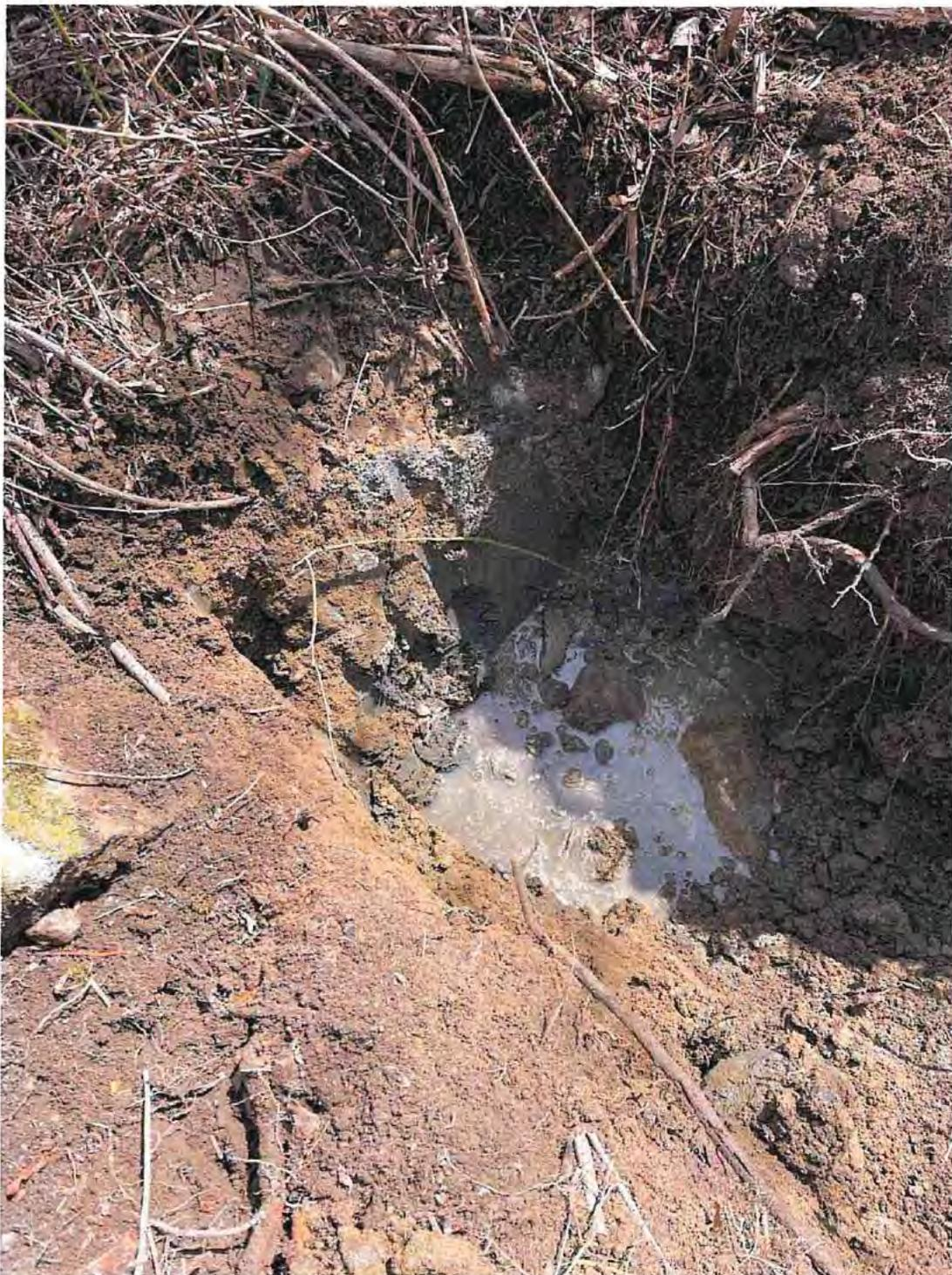
Figure 1: View of test hole #1, groundwater found 3'-6" below the existing top grade.
