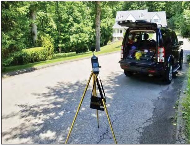
**Photo 3. Sound Meter and Data Recorder**
