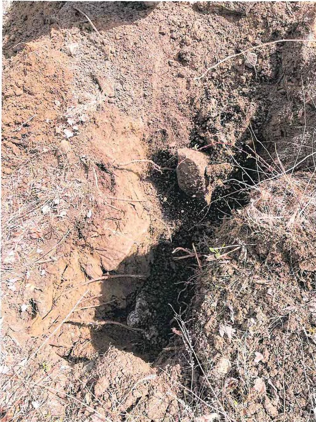
Figure 1: View of test hole #1, groundwater found 5'-0" below the existing top grade.
