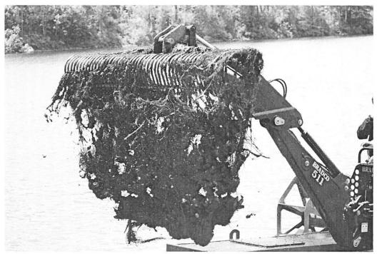
The Hydro-Rake can be described as a "floating backhoe". The equipment can operate in shallow water (<2 feet) and it can work to depths of 12 feet. The Hydro-Rake is successful at removing plants, hummocks, roots, stumps and emergent shoreline vegetation. A hydro-rake is operated from the water to "rake" the sediment layer, collecting plants and detritus with its various attachments.
