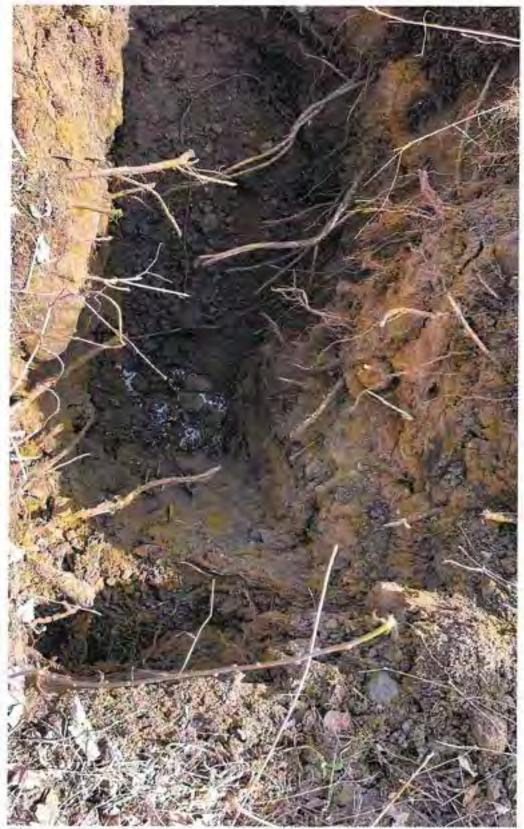
Figure 1: View of deep test hole (Test Hole#1) at 72-inches deep and the 30-inch pvc pipe used to determine the infiltration rate.
