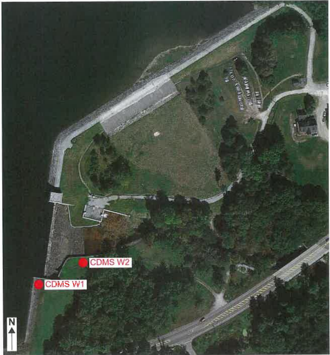
West Branch Dam – Proposed Boring Layout Plan
