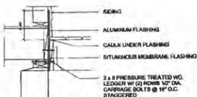
FLASHING DETAIL NOT TO SCALE
