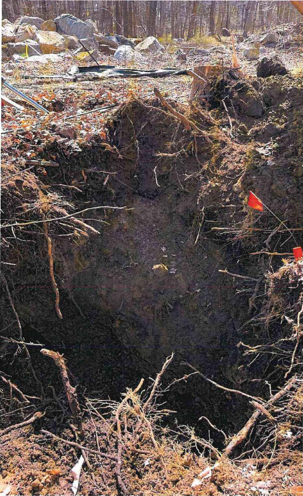
Figure 2: View of the soil profile (Test Hole#1).
