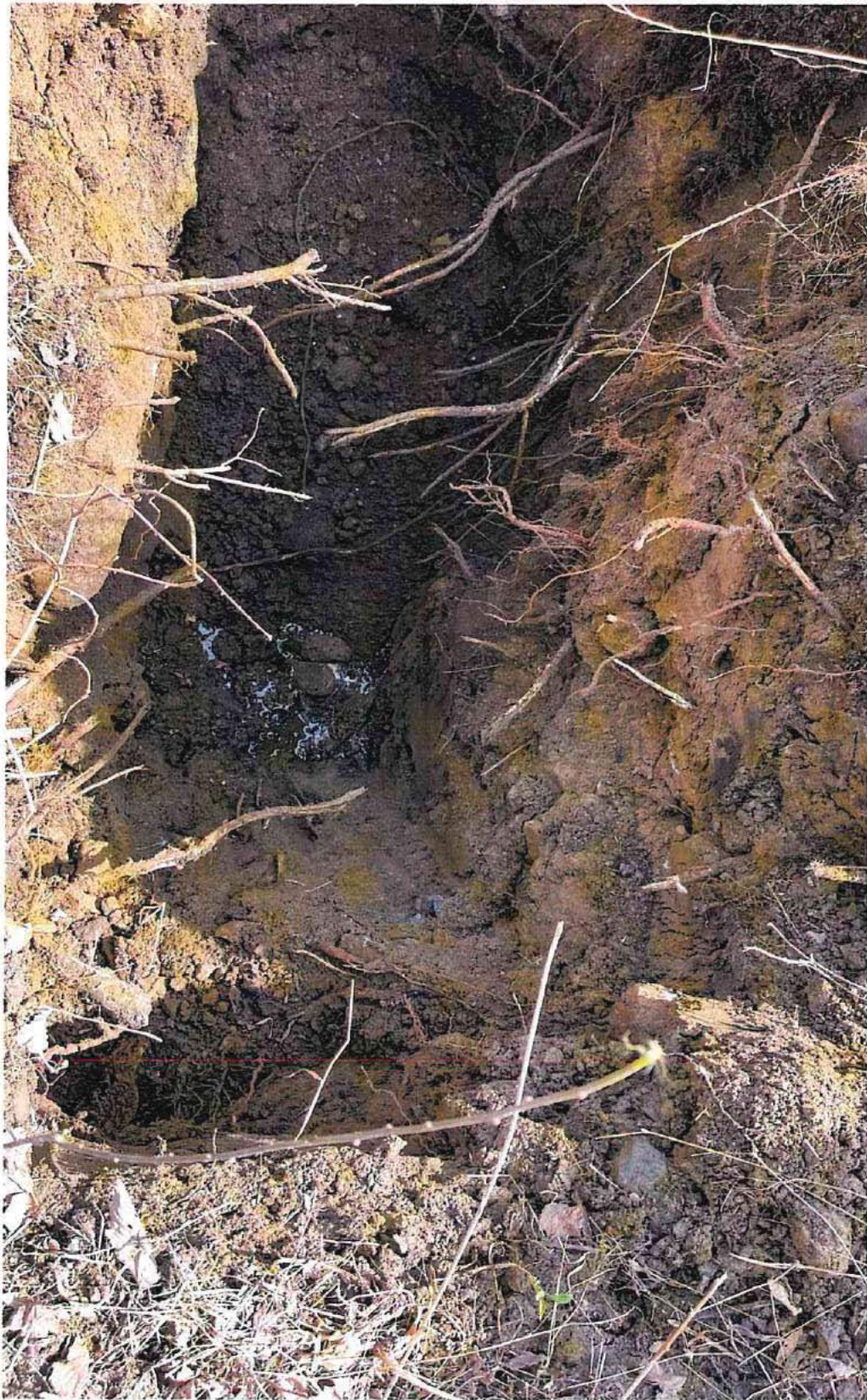
Figure 1: View of deep test hole (Test Hole#1) at 72-inches deep and the 30-inch pvc pipe used to determine the infiltration rate.
