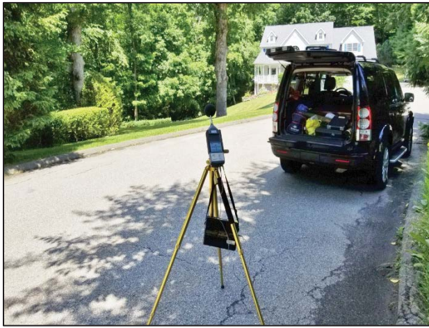
Photo 3. Sound Meter and Data Recorder
