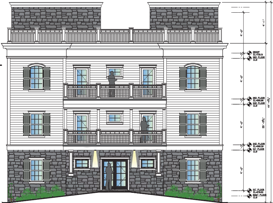
2 REAR ELEVATION (SOUTH SIDE) SCALE: 1/4" = 1'-0" NOTE:
