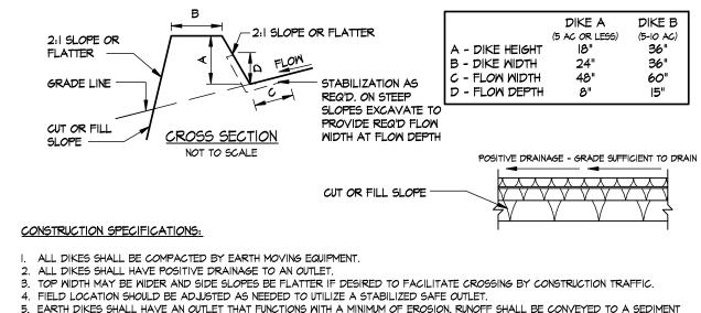
5. EARTH DIKES SHALL HAVE AN OUTLET THAT FUNCTIONS WITH A MINIMUM OF EROSION, RUNOFF SHALL BE CONVEYED TO A SEDIMENT TRAPPING DEVICE SUCH AS A SEDIMENT TRAP OR SEDIMENT BASIN WHERE EITHER THE DIKE CHANNEL OR THE DRAINAGE AREA ABOVE THE DIKE ARE NOT ADEQUATELY STABILIZED. 5. STABILIZATION SHALL BE: (A) IN ACCORDANCE WITH STANDARD SPECIFICATIONS FOR SEED AND STRAW MULCH IF NOT IN SEEDING SEASON, (B) FLOW CHANNEL AS PER THE CHART BELOW:
