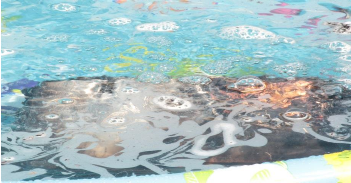
Figure 26 Submerging batteries in water resulted in cooler temperatures, but slow shorting and persistent CO generation (bubbles).
