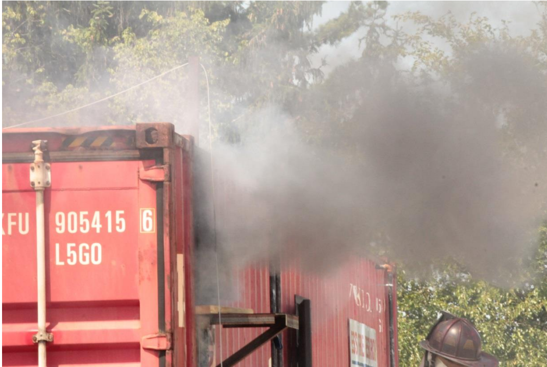
Figure 24 Smoke plume rising through door gaps and out of top vents in the burn container.
