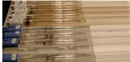
Figure 1: The four top non-OEM lamps (white ends) show permanent brown discoloration after only 3,833 hours. The four bottom genuine Trojan LP lamps (blue ends) are clear and maintain proper levels of UV output.
