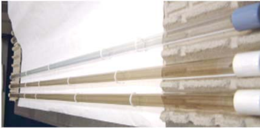
Figure 2: The two bottom non-genuine test lamps show permanent brown coloration after 3,833 hours. The top genuine Trojan low pressure lamp is clear and maintains proper levels of UV output.
