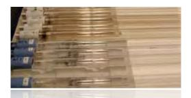
Figure 1: The four top non-OEM lamps (white ends) show permanent brown discoloration after only 3,833 hours. The four bottom genuine Trojan LP lamps (blue ends) are clear and maintain proper levels of UV output.
