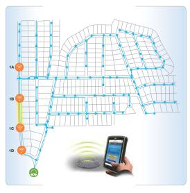
iTracking analytics immediately discover that micro basin 1C, comprised of adjacent manholes 1B - 1C, is contributing 75% of the l&I within all of mini basin 1.
