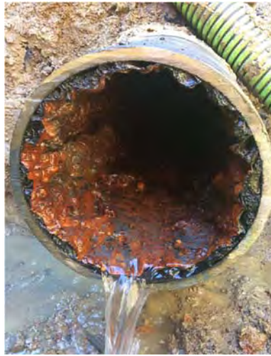
Figure 2-10: Coupon of Tuberculated Pipe on Seminary Hill Road 7
