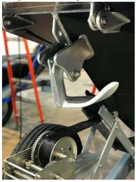
Figure 3: Bow Pulpit for Anchor
