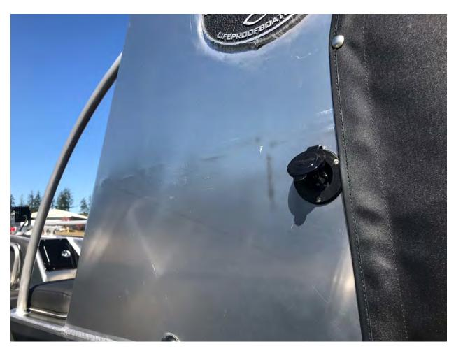
With a battery charger option, we install this simple plug on the side of the console which allows a orange extension cord to plug directly to it when the boat is stored on the trailer and you want to keep the batteries topped off.
