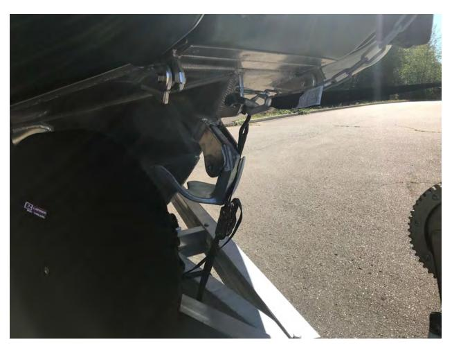
Bow Anchor can be configured in a standard locker or a thru-hull pulpit like shown above.
