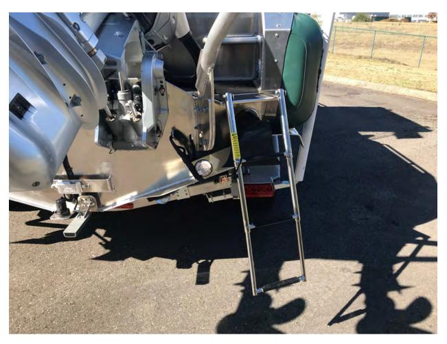
Three or Four Rung Ladder off stern swim deck for easy egress from water and or access to boat even when on trailer.
