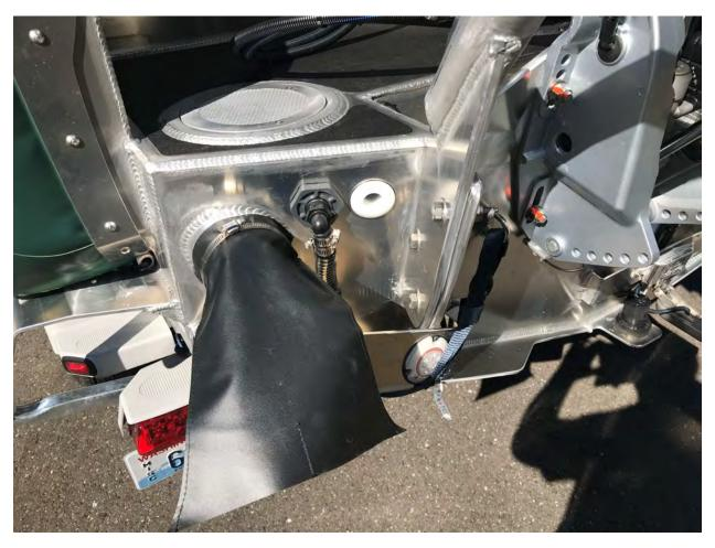
All hull penetrations happen above waterline except for a single drain plug in the boat which is below waterline. All accessories are mounted to exterior brackets / plates off transom.
