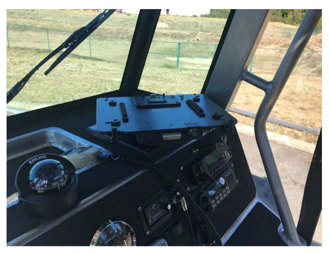
IMS manufactured a simple low-profile swivel for the above laptop docking station.
