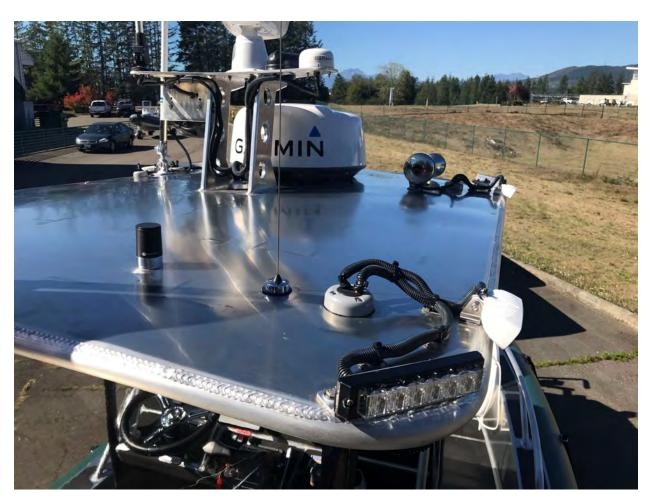
Standard in our hardtop police models is to use corner mounted LED alert lights made by CODE3.
