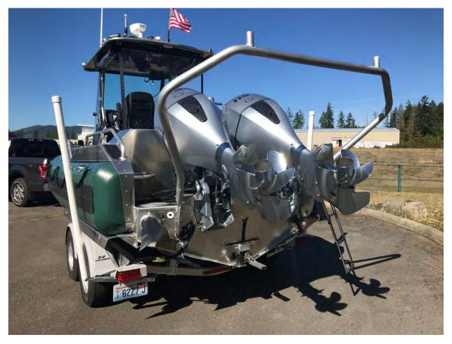
Can be configured with a Single outboard or Twin outboards.
