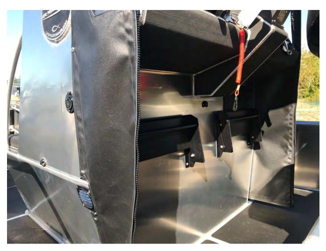
Multiple options available for footrests including these simple fold-up foot-rests mounted to the console.
