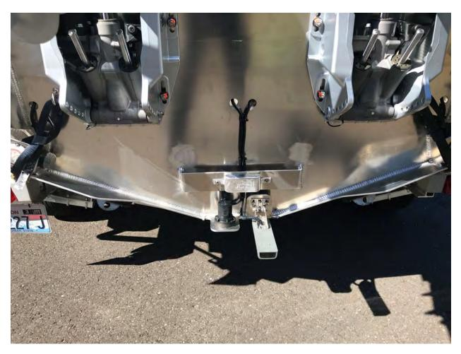
Dual transducer configuration easily adapted for ability to have a high speed chirp transducer with a side-scan transducer in combination.
