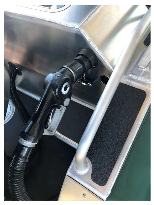
A direct fueling point for the tank is located at the STBD aft corner of the rigging locker.
