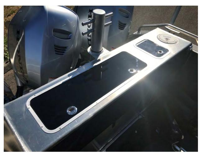
Rigging lockers are customizable in layout based on what is ordered. The lower half is typically dedicated to rigging, and the top half can be configured with storage or other options including a walk-thru transom door or a bench seat.
