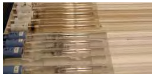
Figure 1: The four top non-OEM lamps (white ends) show permanent brown discoloration after only 3,833 hours. The four bottom genuine Trojan LP lamps (blue ends) are clear and maintain proper levels of UV output.
